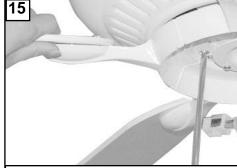
Check the motor for plastic shipping stabilizer tabs, and remove them if they are present. The screws, washers, and motor pads are preinstalled to the blade holders. Attach blade assembly to motor and tighten screws securely.
